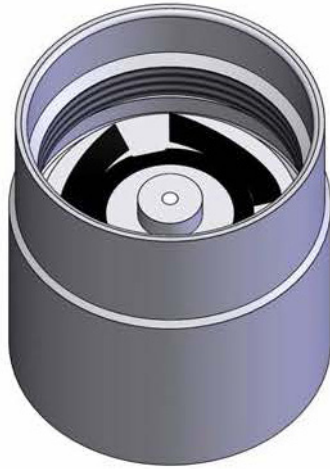
Figure 2: Finger Spring Washer Installation
