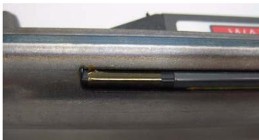
2.4 Install the 2 O-rings (item #10) to the Detonator Housing (item #11), and then attach the housing to the PX-1 Carriage (item #7) using the 2 Pan Head Screws (item #9).
