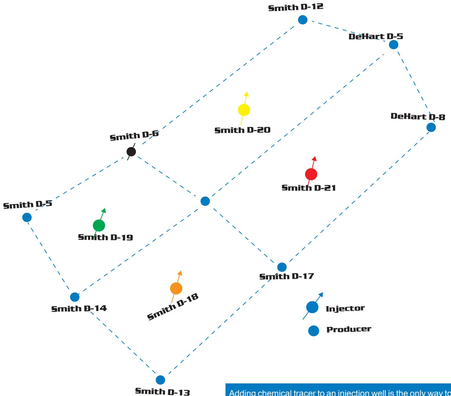
Adding chemical tracer to an injection well is the only way to differentiate between injection water and formation water, and between other injectors in the field. By tagging each injector's water with a unique tracer fingerprint, we are able to quantify an injector's support of an offset producer.
