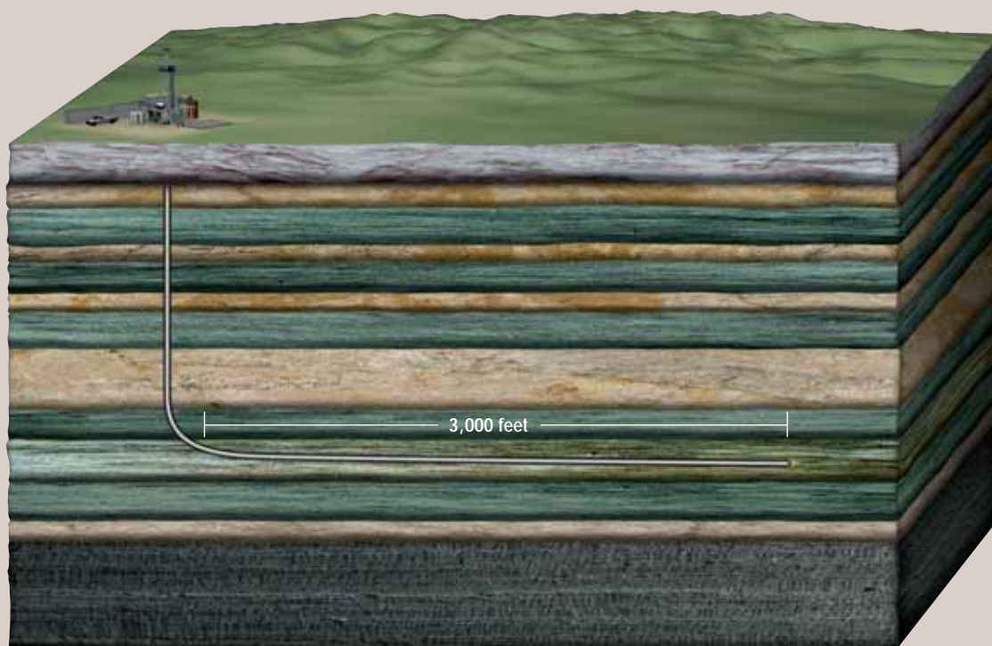
Figure 3. Wells are turned to horizontal in the Barnett Shale formation for maximum penetration and exposure of the wellbore to the organic-rich and gas-prone rocks within the shale layer.
