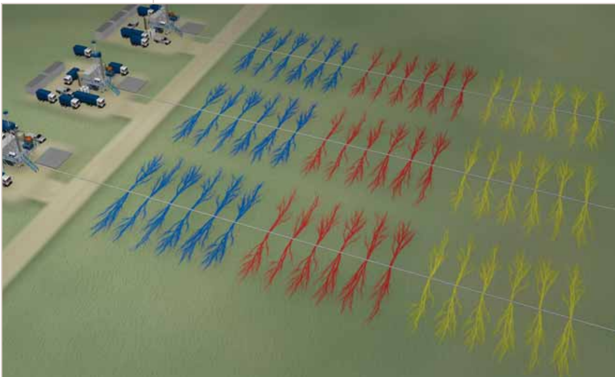
Figure 7. Multi-staged simul-fracs expand the surface area of the shale that can freely flow natural gas into the fracture system.
