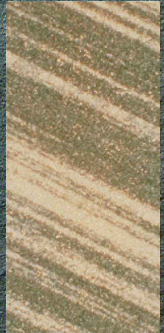
Figure 2. Sandstone core slab.
