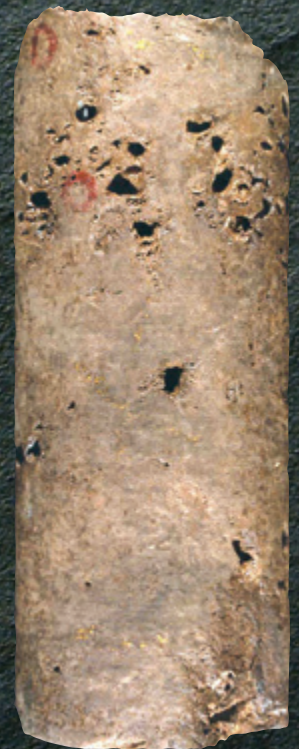
Figure 3. Carbonate core sample.
